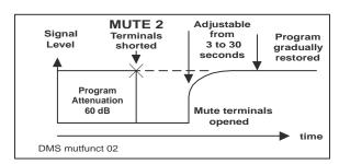
Fig. 17C - M 2 Function Timing Diagram
